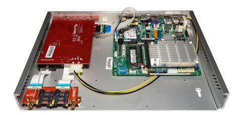
If mounting an additional 2GSM module use the pre-attached SIM and antenna cables.
