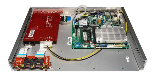
**Step 6:** Push the top cover back in and place the back plate back on. Insert the 4 SIM holders into the GSM\_Extension Kit and attach the antennas. Done!
