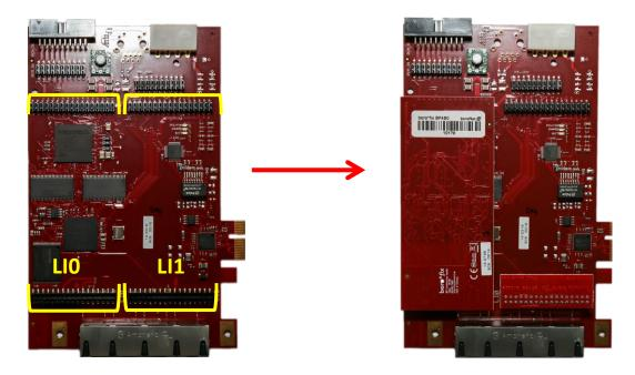
The PCIe-Card has to be placed with the modules face-down on the 3 bolts.
