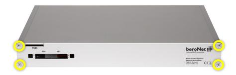
**Step 2:** Remove the top cover by pushing it towards the back of the appliance.
