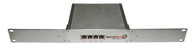
In order to attach the 19" brackets to the gateway use the 3 mounting threads on the sides of the gateway.
