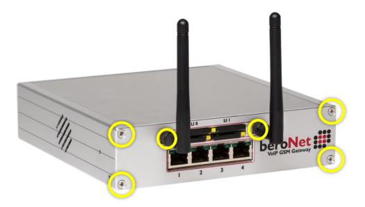
In case of a 2GSM beroNet Gateway the 2GSM module is placed on LineInterface 1 (LI1) because it has a built-in BFBridge. This allows you to place a 4 port module without using an additional BFBridge.
