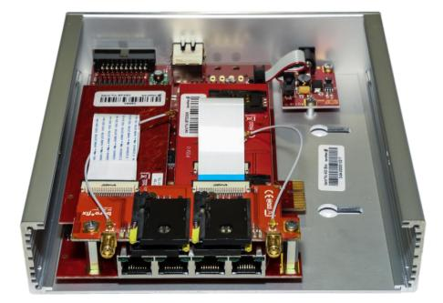
In case of upgrading the GSM Gateway with an additional 2GSM module it has to be connected with the GSM\_Extension Kit. Use the pre-attached cables on the GSM\_Extension Kit.
