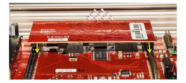
In case of a single 4 port module it is recommended to use the included BFBridge. Placing the BFBridge on the LineInterface 1 (LI1) will unlock the two additional RJ45 ports.
