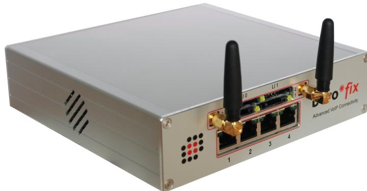
Connect your berofix Gateway to your local area network (LAN) or connect it directly to your computer using a cross-over cable. After that power-up the device.
