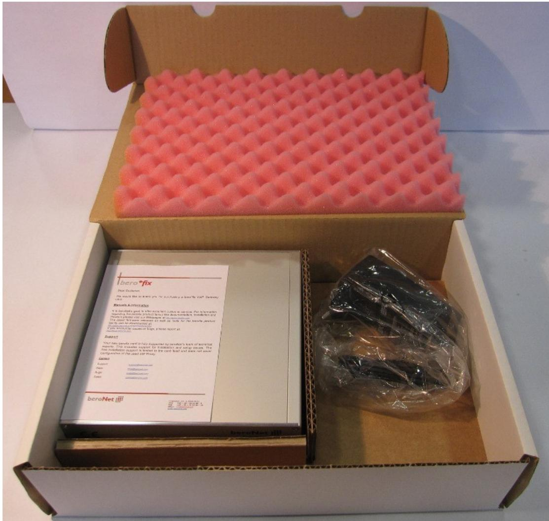
The beroFix Box contains the gateway itself and the Power Supply. The Gateway contains no modules, these are shipped separately.
