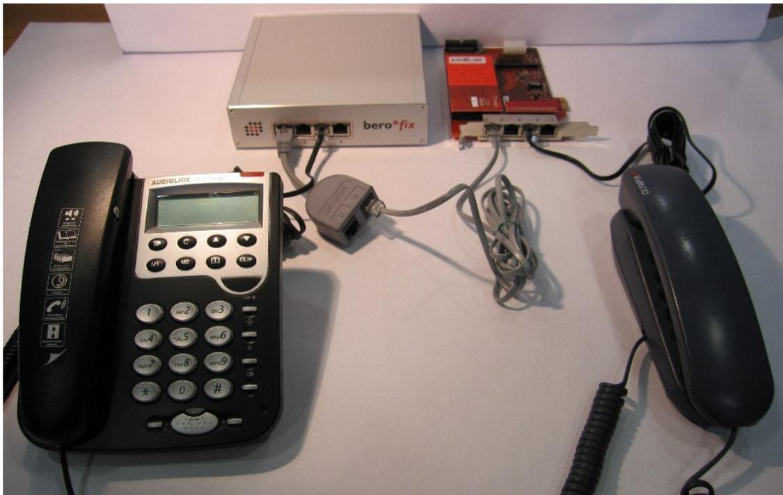
The connection of all devices and cables can be seen above. Make sure to use the beroNet T-Adapter on the PSTN simulator. You can see that port 1a of the PSTN simulator is connected to port 1 of the PBX beroFix. Port 3 of the PSTN simulator is connected to an analog phone. Port 3 of the PBX beroFix is also connected with an analog phone.
