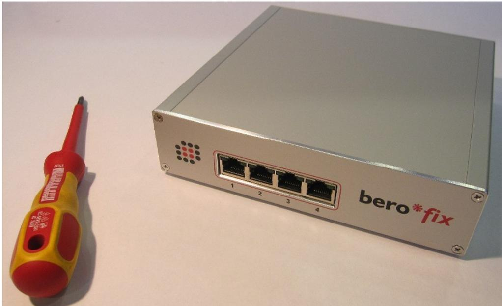
To open the box, just unscrew the four screws at the front side of the gateway and slide out the top like in the following picture.
